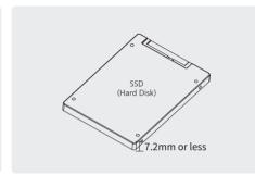
1. Loosen the captive screws and remove the rear cover. | 2.5 inch SATA hard drive up to 7.2mm high
